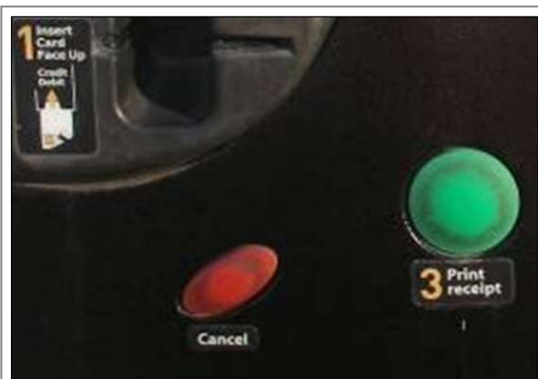
Chicago: Besides different colors, the buttons have different shapes and labels.
