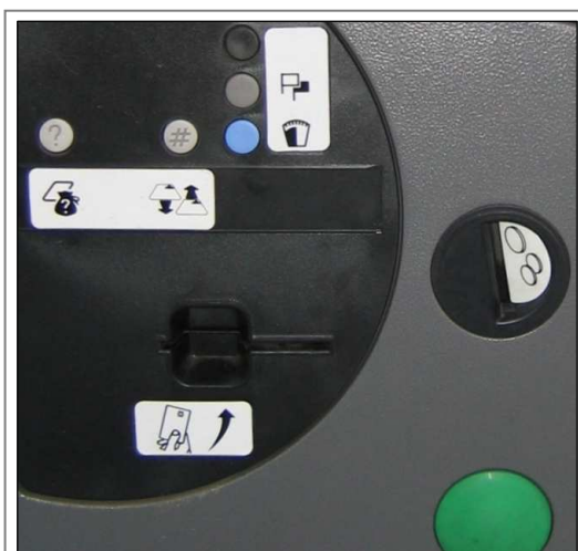
Munich: size of the blue 'add time' button is much smaller than the green 'confirm' button.
